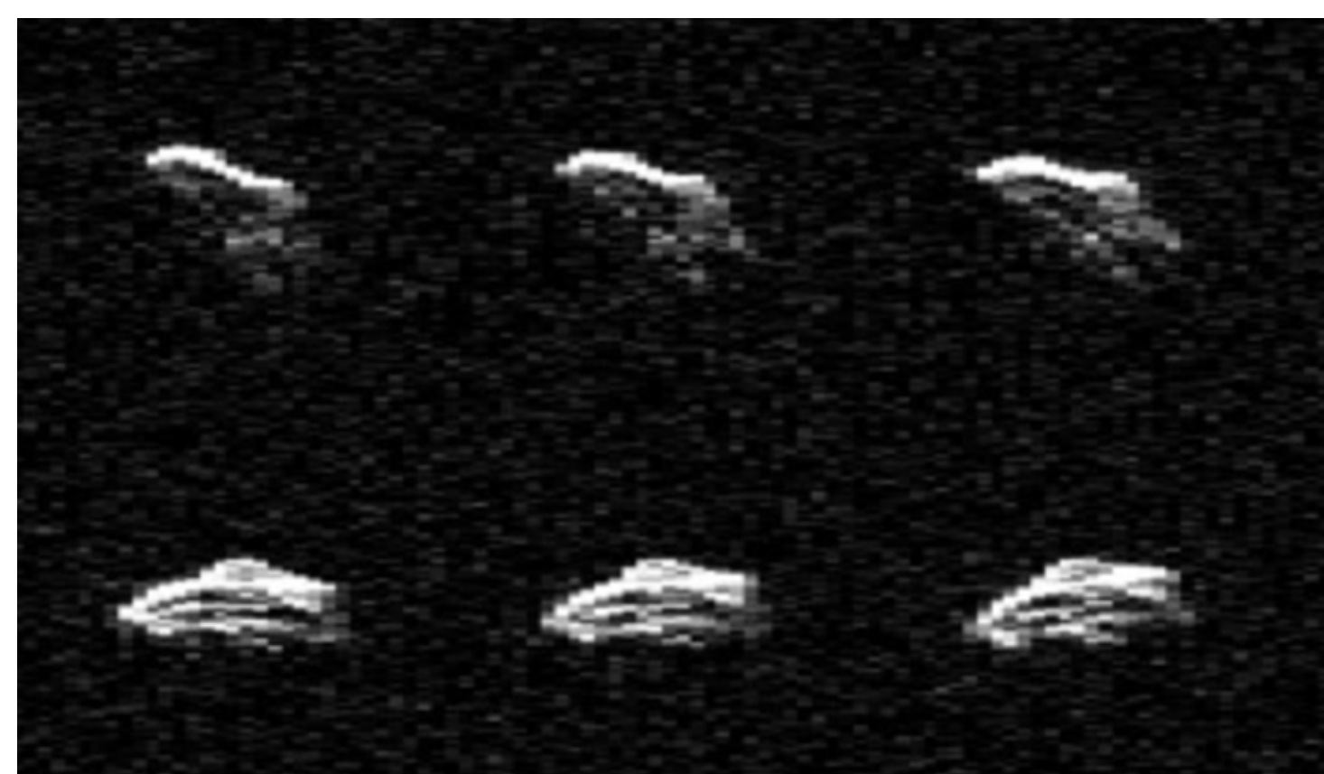
Figure 8 - Delay-Doppler images of 2011 UW158 obtained on 2015 July 18 from Goldstone using SS-14 to transmit and Green Bank Telescope to receive. Resolution is 7.5 \text{ m} \times 5 \text{ Hz} . Range increases down and Doppler frequency increases to the right. The images span a little more than 1 rotation of the object (Goldstone Radar Team; Naidu et al., 2015).
